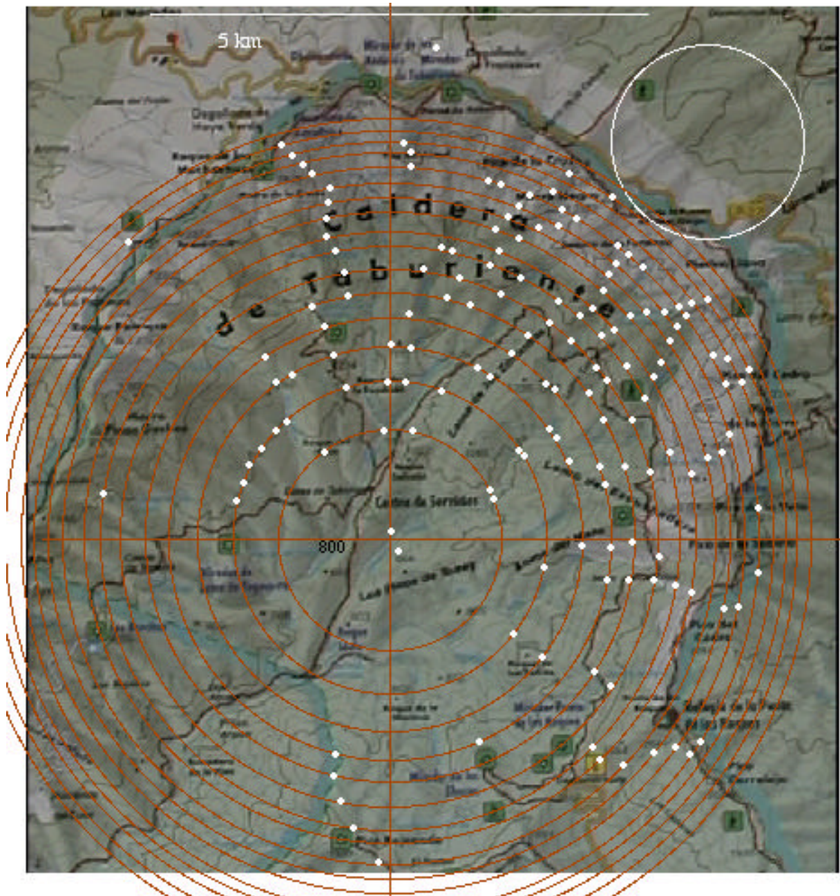
Figure 4: Altitude contours of a hemispheric dish fitting optimally in the Caldera, showing intersections (white dots) with ground contours which are possible locations for mirrors. The sphere's radius is 6500m and the altitude spacing of contours is 100 m. The array can span about 7500 m in the North-South direction, but the effective aperture size usable on a given star will be smaller than 2400m ( the white circle corresponds to 2,000m), being limited in practice by the feasible size of the focal corrector. The location of the effective aperture varies with declination and the hour angle. The possible co-spherical site for the Euro-50 indicated at top left can be on the outer slope for invisibility from the Caldera. It extends the baselines lengths, especially when observing towards the North, and up to 6,600m when observing at 53° declination. The focus' altitude is 4,050m above sea level, i.e. 1,750 m above the crater's rim at 2,300m. The range of zenith distances accessible is 25° North and South of zenith, covering declinations from +3 to +53°.
